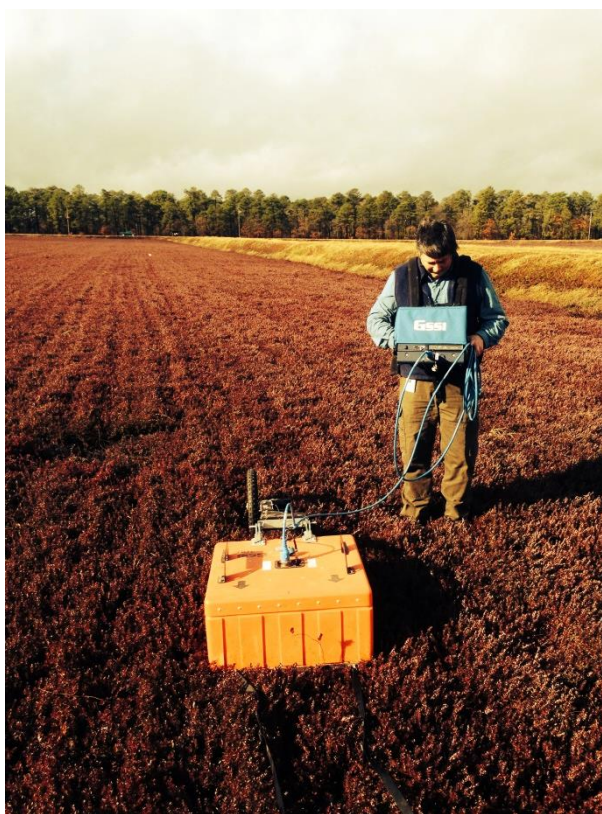
Testing the 200 MHz antenna in a cranberry bog.
